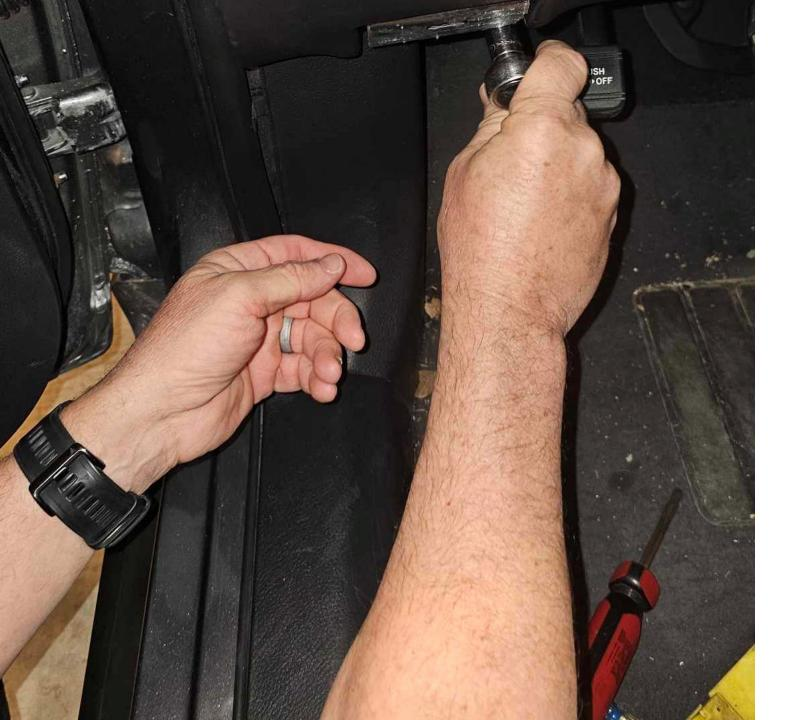
Step2-Remove two 10mm bolts for release lever and let it drop down:
