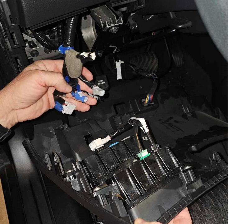
Step4- Remove the connectors on lower console so you can put it aside. Note: there is a connector latch you push down that allows the connector to easily come out. Might need to use small screwdriver to push, my fat fingers had a hard time.
