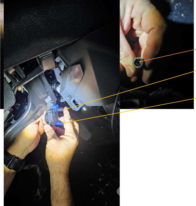
Step8-Install new slip gear on actuator shaft.
