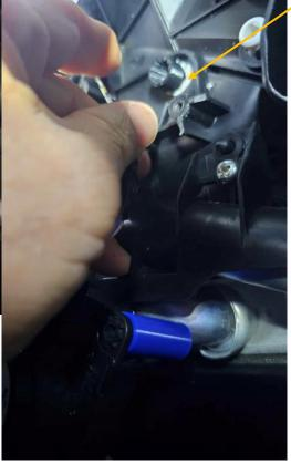
Step 9-Install new receiving spline into stripped spline, on blend door.
