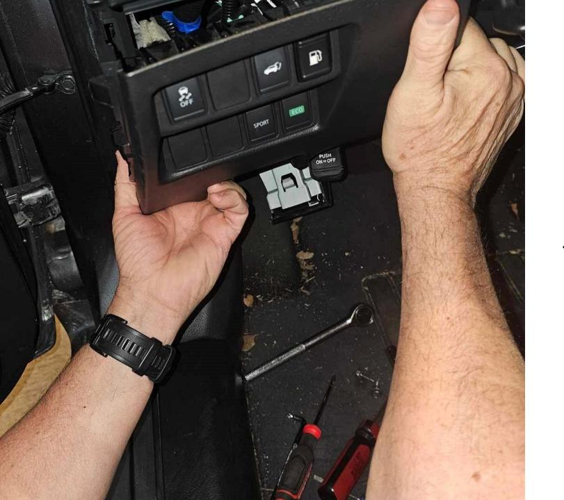
Step3-Remove lower cover, this piece has no bolts and just snaps out. Work its way loose all the way to the center console:
